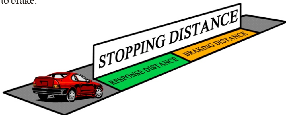
Picture 28 – The TOTAL STOPPING DISTANCE is the sum of Response Distance (Reacting Distance) and Braking Distance:
