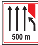
Right lane ends 500 m
