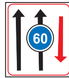
Restriction/prohibition applicable in right lane
