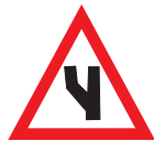
Beginning of dual roadway (to left)
